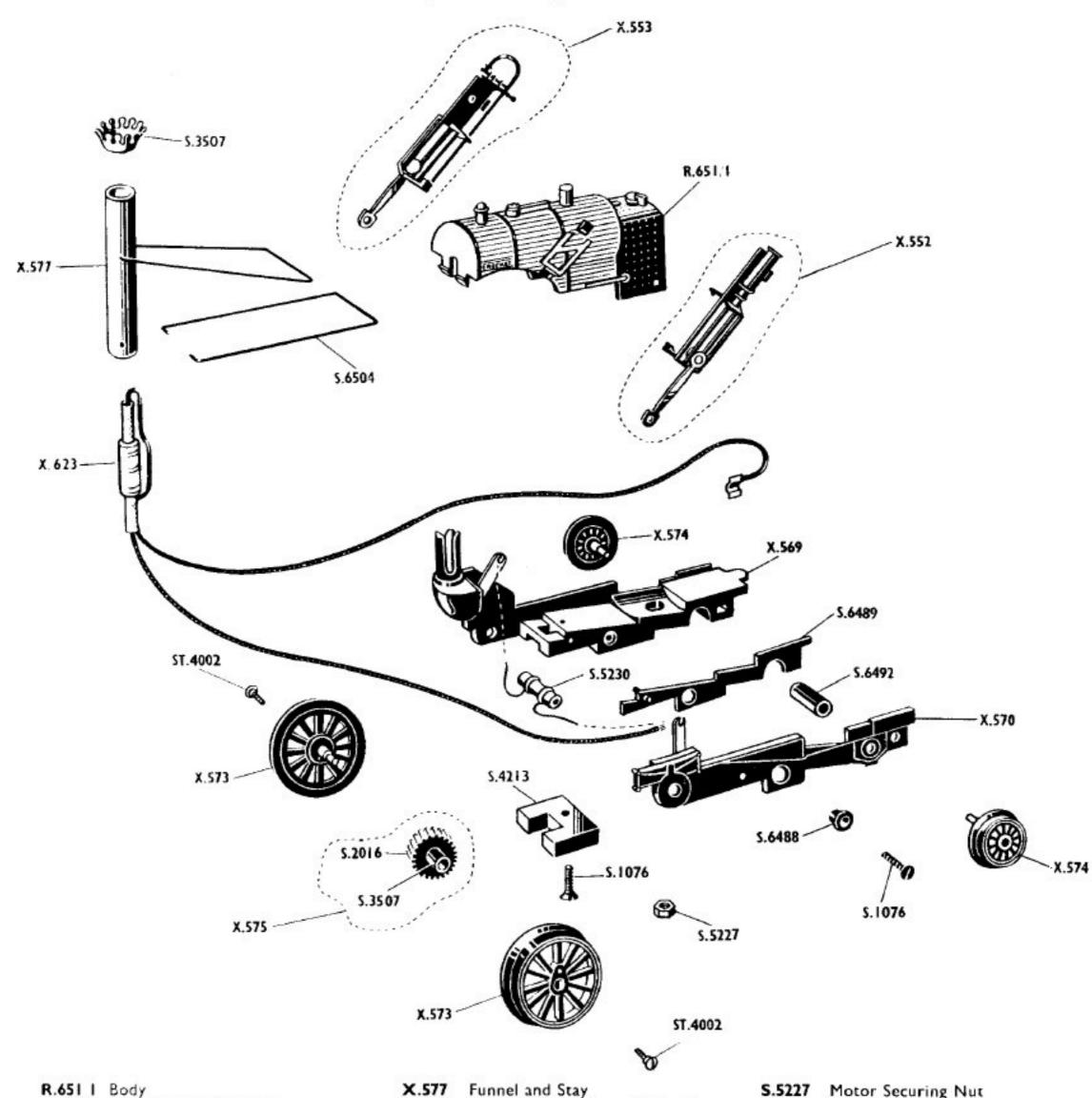
X.552 L H Cylinder Assembly X.553 R H Cylinder Assembly Chassis Assembly X.569 X.570 Side Frame X.573 Driving Wheel Trailing Wheel X.574 X.575 Worm Wheel and Axle
